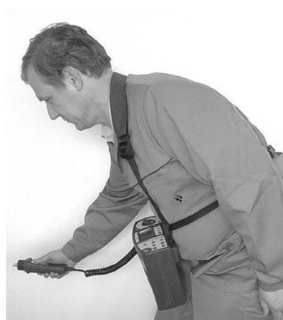
*The instrument is hung around operator's neck and fixed to his body with back belt - stable position.*
